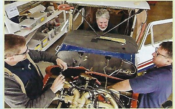
Chuck, Jim, and Dale work together to install the new Continental IO550 engine.
